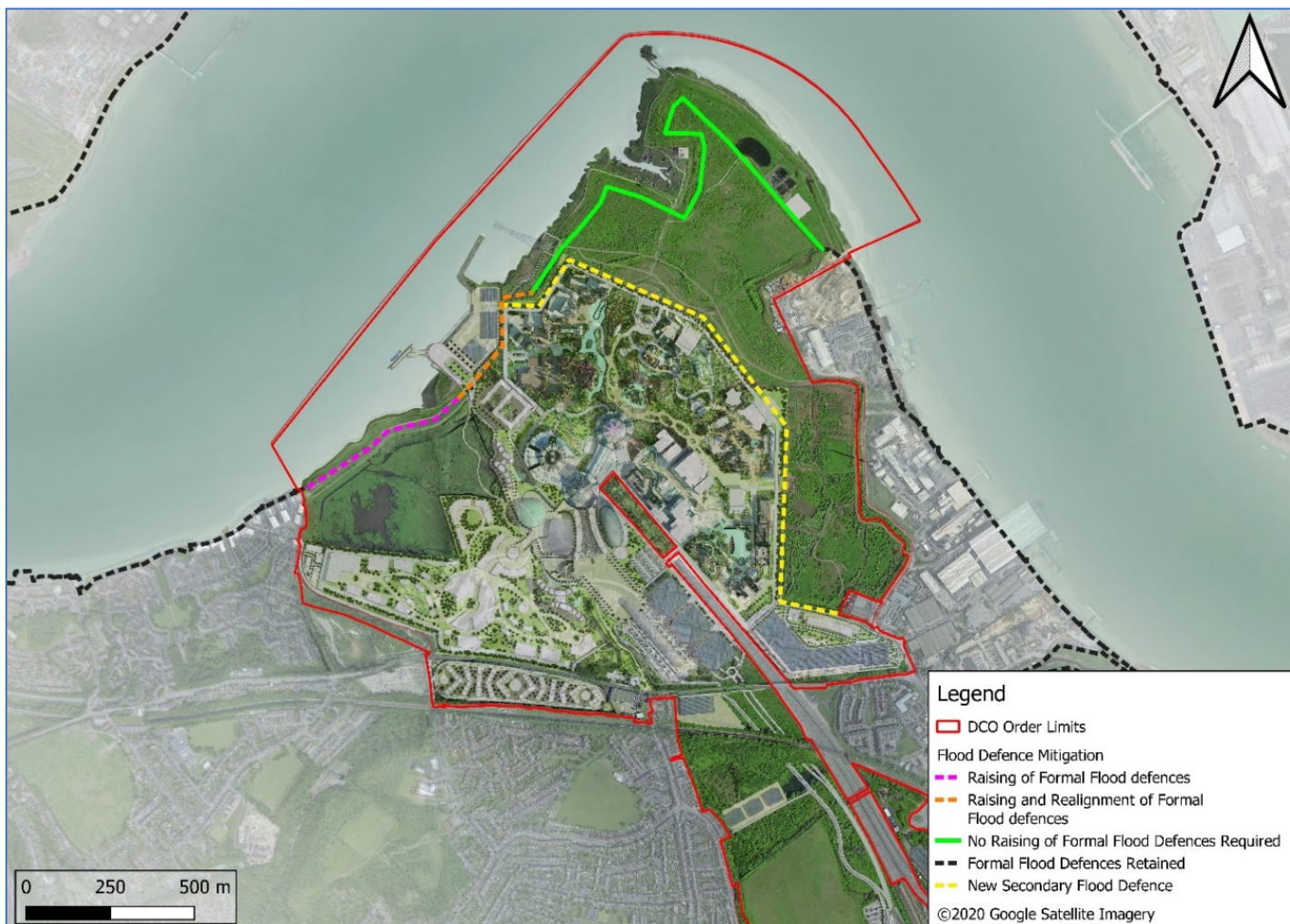
Figure 17.33: Proposed mitigation measures to provide the required standard of protection to the site from tidal overtopping.
